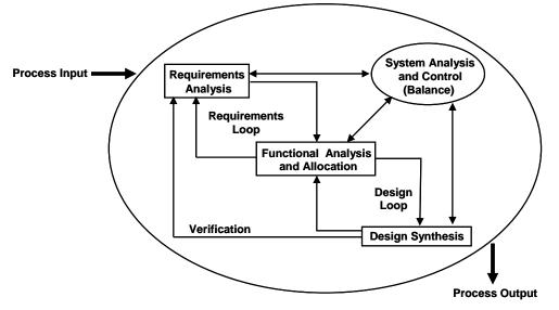
Figure B-1. An Approach for Performing Front-End Systems Engineering
