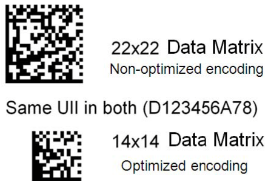
Figure 11. Minimizing Cell Count Through Optimized Encoding
